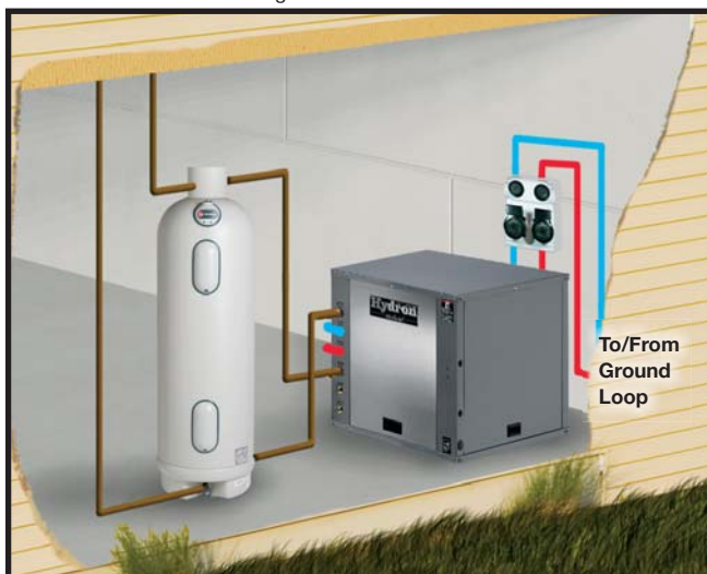
Common Water-to-Water geothermal installation.
